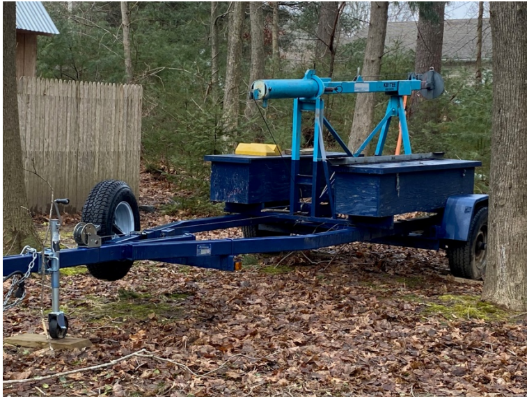
My ham radio tower trailer 35 feet tall when set up KB1TEE
