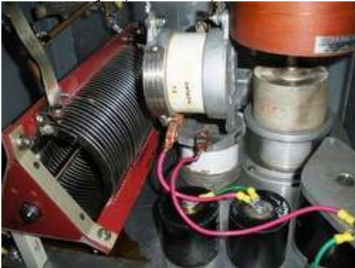
The plate tank circuit in the WH2XBA/1 VLF transmitter. [Bob Raide, W2ZM, photo]
