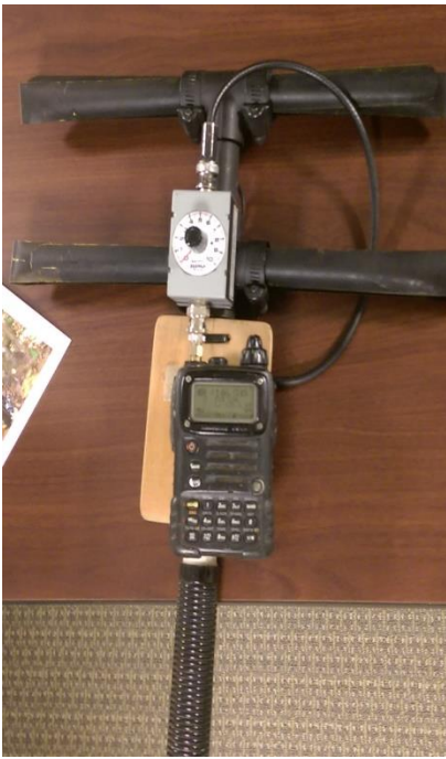
In the Photos Above Left: At our February 2016 MARA Meeting , Richard – AG1B gave a presentation of his Fox finding equipment which includes a close up of the Antenna / Attenuator box and his Baofeng Transceiver typically set to 146.535 MHz in order to search for the Fox! Above Right: Richard – AG1B demonstrates his Foxbox in operation with Phil – N1XTB and Jeff – N1ZZN looking on! Not in the photos are: Philip – SWL and Loren – N1IQI Photos by Barry – N1EZH
