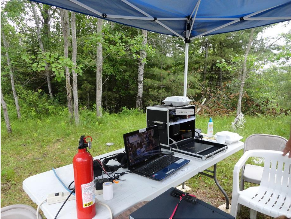
My portable rig Yaesu 7800 dual band 2m 70cm sec 1200 power supply my gateway computer with Squil field day logger
