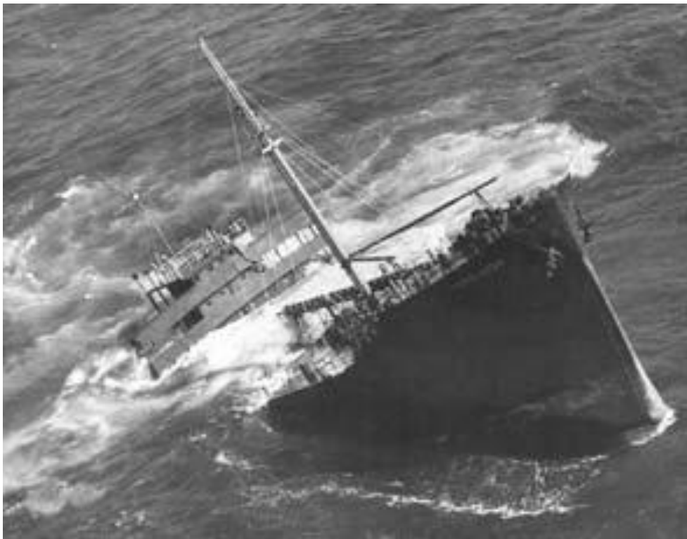
This is the actual tankers bow section that broke free from the ship. This section was later refloated and taken to be scrapped in Delaware
