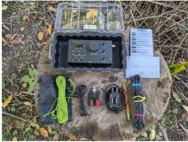
The radio is an Elecraft KX1. It's a four band radio with the internal ATU. Powering it are six AA Lithium Ion batteries.
