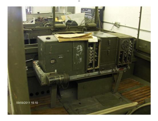
The SCR-508 radio was a mobile Signal Corps Radio used by the U.S. Army during World War I
