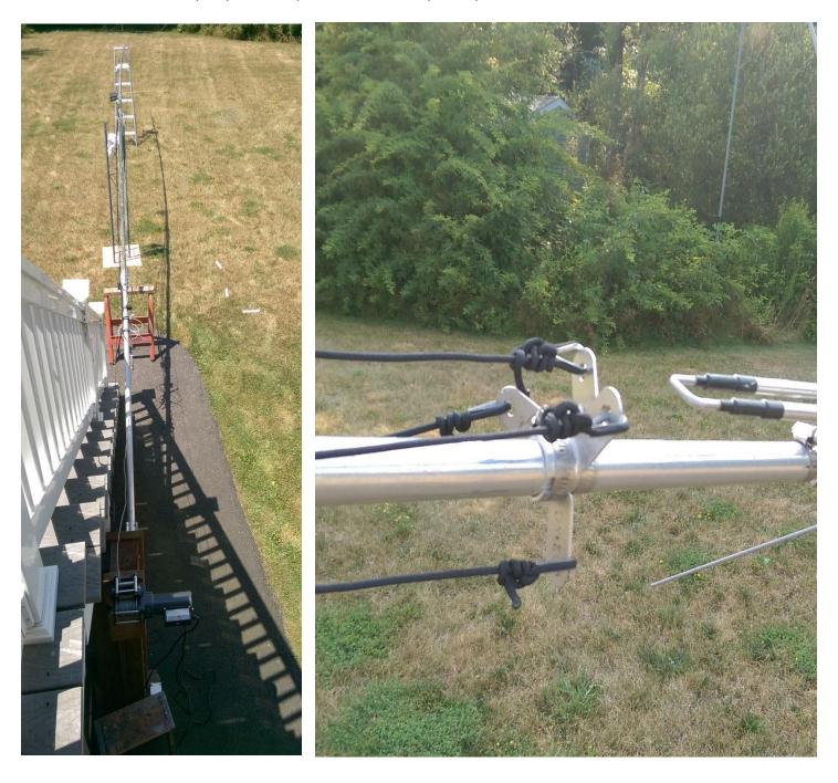
Below: Mast, Cushcraft R7 Vertical and SPI-RO-D56 back up in the air with the 4 Guy Ropes in place to Stabilize the top of the Antenna! There are also 3 Guy Wires on the Military Mast Poles as well!
